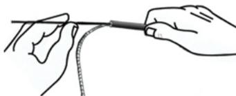
6. Once the cord has been threaded through all of the poles, detach and withdraw the wire. Stretch the cord 16cm out of the pole and tie a knot.
