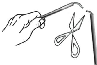
1. Remove the old shock cord to separate the poles
