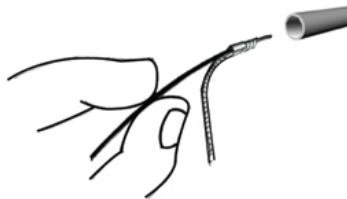
5. Insert the wire with cord into the first pole and thread through.
